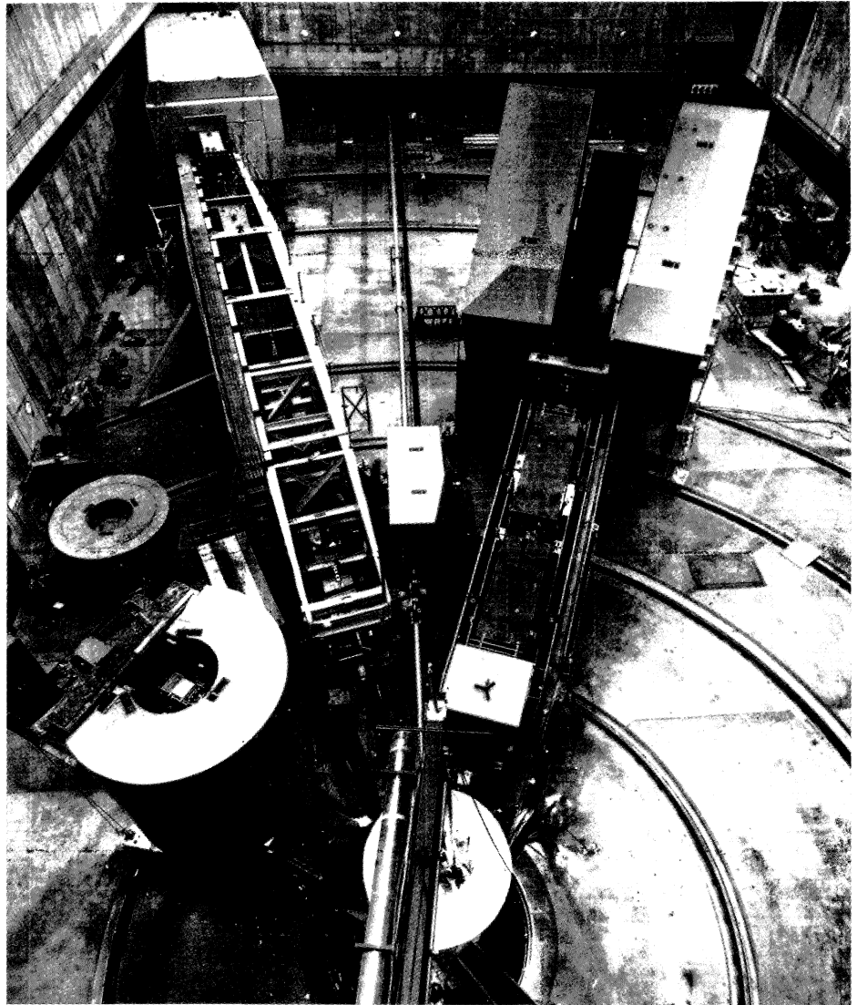
The big spectrometers at End Station A of the Stanford Linear Accelerator Centre (SLAC) in 1967: right of the beamline, the 8 GeV spectrometer, and on the other side its 20 GeV and 1.6 GeV (extreme left) counterparts.
